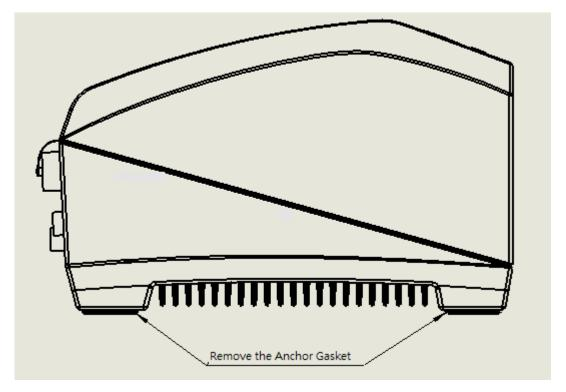
Remove Anchor Gasket by Hand
