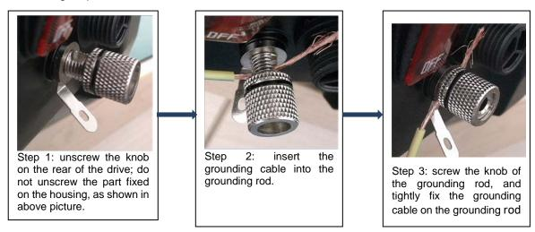
Or directly solder the grounding cable on the grounding rod.
