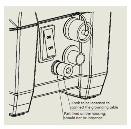
G100-2J/ G300-2J are equipped with grounding rod. The pump could be grounded well through the grounding rod. Grounding the pump will prevent the misoperation and damage because of the electromagnetic interference.
