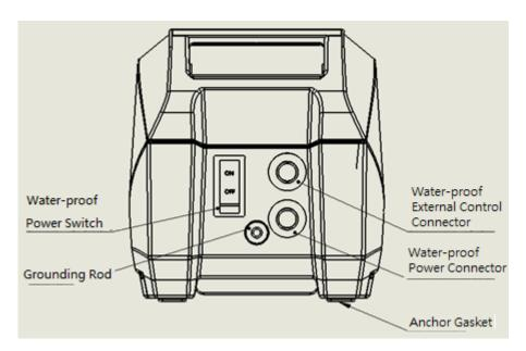
"Anchor gasket" is the default configuration of the drive, mainly used for buffer and vibration attenuation. When it is needed to fix the drive on an external platform, an "adapter bracket" should be selected. Please refer to chapter 3.1.2, "Fixing of G100-2J/ G300-2J", for removing the "anchor gasket" and mounting "adapter bracket".
