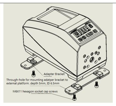
Fixing of Adapter Bracket (Optional)
